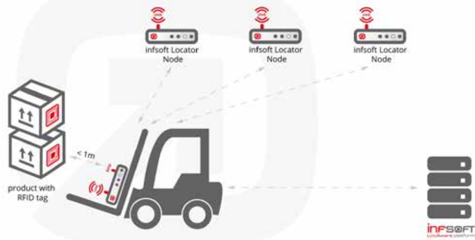
combination of RFID and UWB for identification and localization of goods
