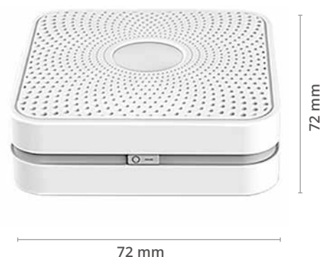
insoft Locator Beacon with dimensions
